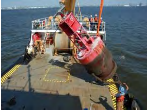
Figure 9-3 Centering the Buoy on the Deck
