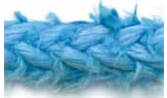
Severely abraded rope.
