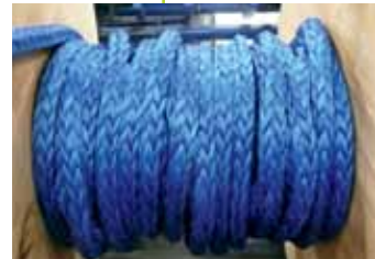
CROSS WINDING Level Layer
