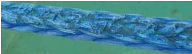
Melting damage on AmSteel®Blue.
