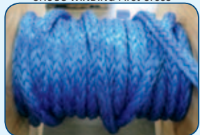
CROSS WINDING Second Cross
