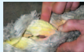
Fig. 2 Inspect for internal abrasion.
