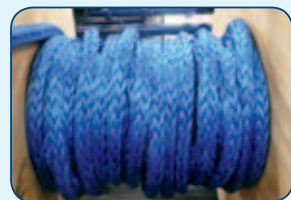
CROSS WINDING Level Layer
