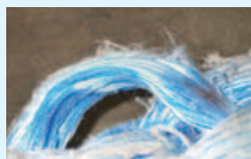
Fig. 1 Inspect for internal abrasion.
