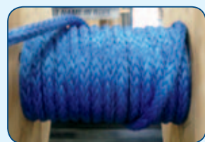
CROSS WINDING First Cross
